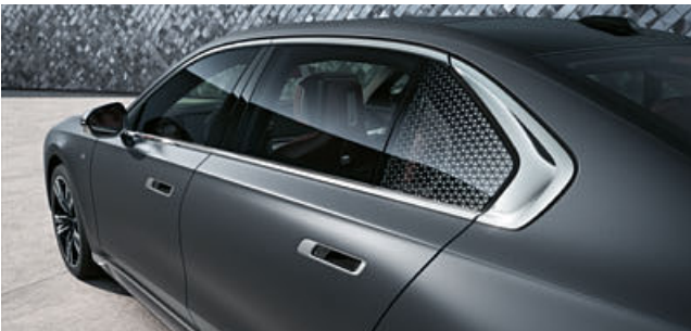
The Sun protection glazing for the rear window and tinted rear side windows reduces unwanted warming of the interior.
