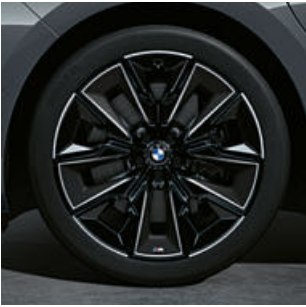
21" M aerodynamic wheels 909 M Multicolour 3D buffed with mixed tyres, gloss-lathed, wheel size front 9J x 21 with 255/40 R21 tyres, wheel size rear 10.5J x 21 with 285/35 R21 tyres. 3
