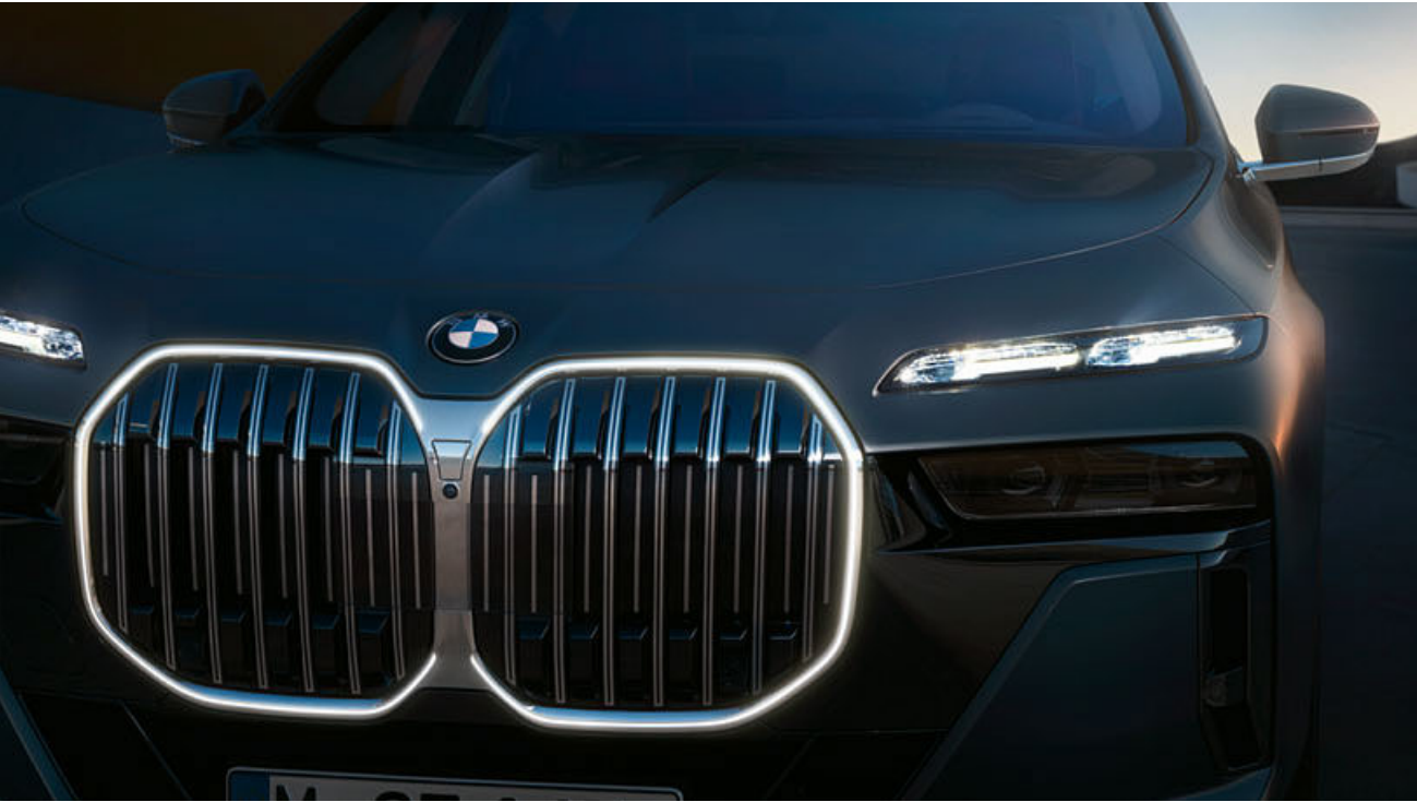
Visual highlight on the exterior: contour line lighting impressively showcases the BMW kidney "Iconic Glow" – both when the vehicle is at a standstill or while driving. LED elements feed a fibre-optic conductor integrated into the kidney frame, which evenly highlights the kidney outlines. When deactivated, the technology is not visible.
