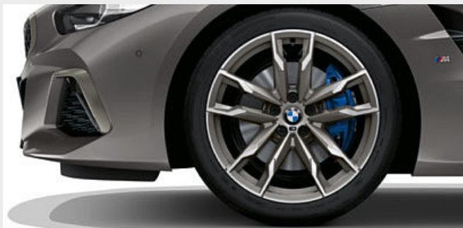
□ 19" M light alloy wheels Double-spoke style 800 M in Bicolour Cerium Grey matt with mixed tyres, burnished, front wheel size 9J x 19, 255/35 ZR19 tyres, rear wheel size 10J x 19, 275/35 ZR19 tyres. 5
