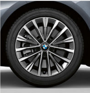
□ 17" light alloy wheels Multi-spoke style 547 Ferric Grey metallic, gloss-lathed, wheel size 7.5J x 17 with 225/45 R17 tyres.¹
