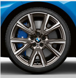
□ 19" M light alloy wheels V-spoke style 557 M Bicolour Cerium Grey metallic, wheel size 8J x 19 with 235/35 R19 tyres.⁴
