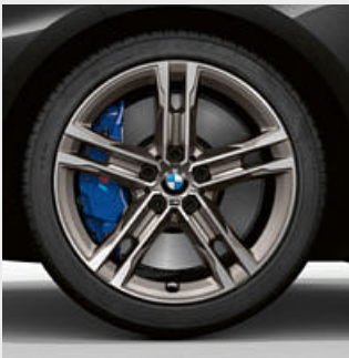
■ 18" M light alloy wheels Double-spoke style 556 M Bicolour Cerium Grey matt, gloss-lathed, wheel size 8J x 18 with 225/40 R18 tyres.⁴
